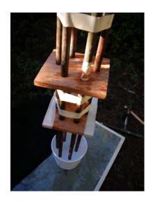
Firm up the unit with tape. Check to see that everything is lined up, and the unit stands up. If you made the top board longer for clamping to a table or whatever to suspend the unit in the bucket, get that set up now also.
