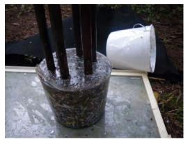
Here is a shot of the piece after pulling it from the mold bucket. This one got mixed a little too hot and the bucket started to melt. You can mist it with water to cool it down, but too much water too fast will make it crack. If you get cracks they can be filled later if you want.
