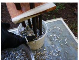
Fill the bucket around the pipes with course metal. If you only have fine or powdered metal then you will need to mix it into the resin first, then pour the mixture into your mold. With the course metal you can pour the resin after you pack the mold.
