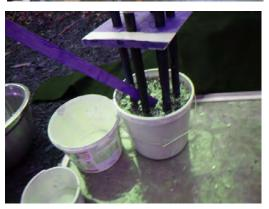
Tamp down the fine bits of metal with a stick or whatever to get all the metal wetted out. You want as much metal in there as possible. The slower the resin mix, the more time you have to pack the metal in and for the brass to sink to the bottom. You can also add other stones. There is peridot mixed in this one in addition to the quartz crystals in the pipes.
