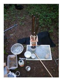
Here is a shot of the unit filled with resin and metal ready for the resin to kick.
