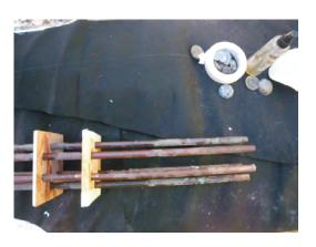
Match up the second board to the first like when they were clamped together. Spray oil was used here to slide the pipes easily in the wood. Lay the unit on the flat side of the boards that you lined up in the clamping step, and get the unit symetrical. You want plenty of pipe showing below the bottom board so that there will be access to the bucket for pouring in the resin and metal later on.
