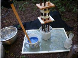
The metal will hold the pipes upright when using short 3' pipes. Mix the catalyst and optional wax into the resin. Use a minimum of catalyst in order to keep the mix from getting too hot when it kicks. This mold held 1/2 gallon. If you have a plastic pitcher to sacrifice, use it. The mixing bucket shown is too small and 3 batches were mixed one after another to fill the mold.
