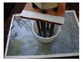
Here there is a layer of metal on top of the sealer coat. If you don't want resin to go in the pipes, rest them directly on to the partialy kicked resin at the botom of the bucket instead. This the point where you would clamp the upper board to a bench to suspend the unit where you want it in the bucket, if you are using that technique.
