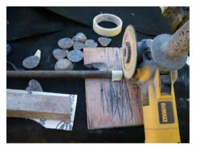
Mark pipes with tape and cut to length. These are 38" long by 1/2" diameter scrap copper pipes. Any metal pipe should work ok. Clean up cuts with sandpaper on a block or a file etc.
