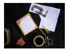
Get 2 pieces of wood, foam board or similar of a size that fits the print-out with room around it. You can make one of them extra long and use the excess to clamp the unit to a table thus suspending it in the bucket exactly how you want it.
