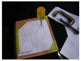
Mark the center of all 6 circles with a sharp object. This will guide your boring bit to the perfect location for accuracy.
