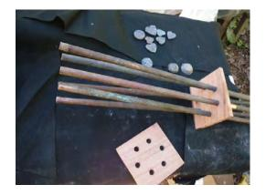
Fit the pipes into the holes on the first board.
