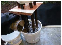
After the resin is in, pour fine metal in now if available. This one has brass and aluminum fine sized metal added.
