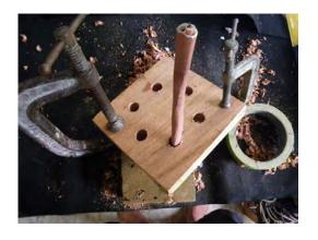
De-burr rough edges with rolled up sandpaper or a file etc.
