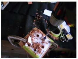
Carefully drill the 6 holes with a boring bit. If using a soft material like foam board, you could cut the holes with an exacto knife or similar. This is a 5/8" bit being used for 1/2" pipe which has an outside diameter of 5/8".
